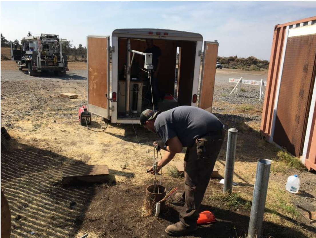
Well logging camera and depth recorder being lowered into the well casing.
