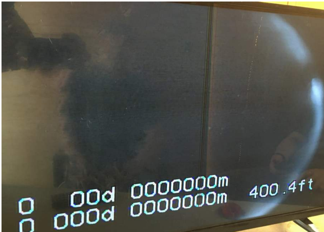
The total well depth was recorded at 400.4 ft bgs.
